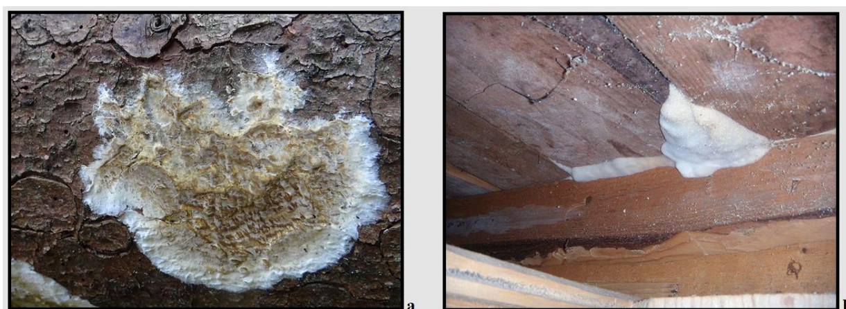
Fig. 2. Example of erosion of an oak beam caused by fungi: a. The initial stage of development of the Coniophora Puteana fungus on a cut tree beam; b. Initial stage of development of Serpula lacrymans fungus on wood.
