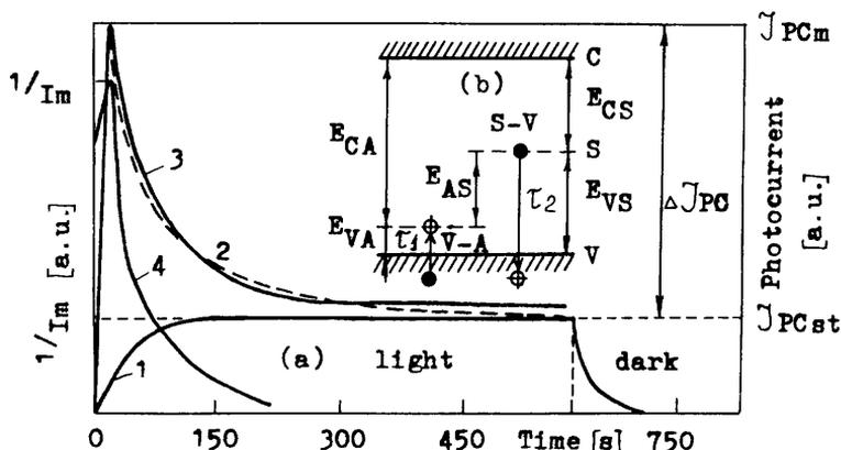
Fig.1. PC decay spectra (a); energy-band diagram of the two-levels model (b).
