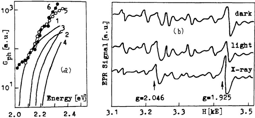
Fig.4. PCCS spectra (curv. for centers 1- $E_{CS} = 2.05eV$ ; 2- $E_{CS} = 2.11eV$ ; 3- $E_{CS} = 2.16eV$ ; 4- $E_{CS} = 2.21eV$  and 5-calculation; 6-experiment) (a); EPR spectra at 77K (b).
