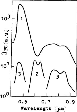
Fig.2. PC spectra without (curv.1) and after preliminary excitation (curv.2) at  $\lambda_{\text{exit}} = 0.525\mu\text{m}$  and curv.3 at  $\lambda_{\text{regist.}} = 0.580\mu\text{m}$
