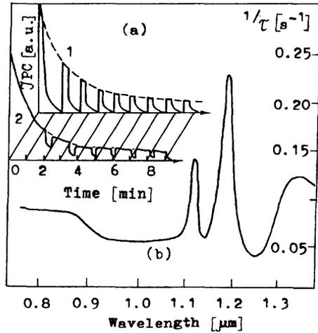
Fig.3. PC decay spectra at  $\lambda_{\text{regist.}} = 0.950\mu\text{m}$  and  $\lambda_{\text{exit.}} = 0.475\mu\text{m}$  (a); spectrum after preliminary excitation at  $\lambda_{\text{exit.}} = 0.490\mu\text{m}$  (b).
