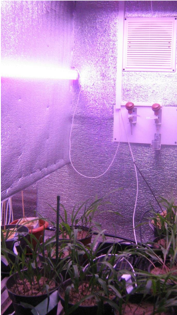
Fig. 1. Phytotron for of the vegetative experience with automated controls
