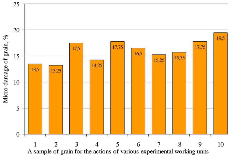
**Fig. 3 - Research results diagram of the grain micro-damage of wheat grain separated by the preliminary threshing device under the conditions of successive setting of experimental working units:**
